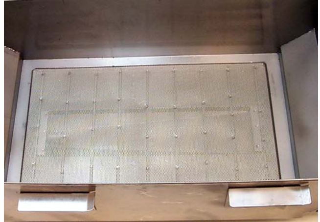
Support grid properly placed in filter pan.
